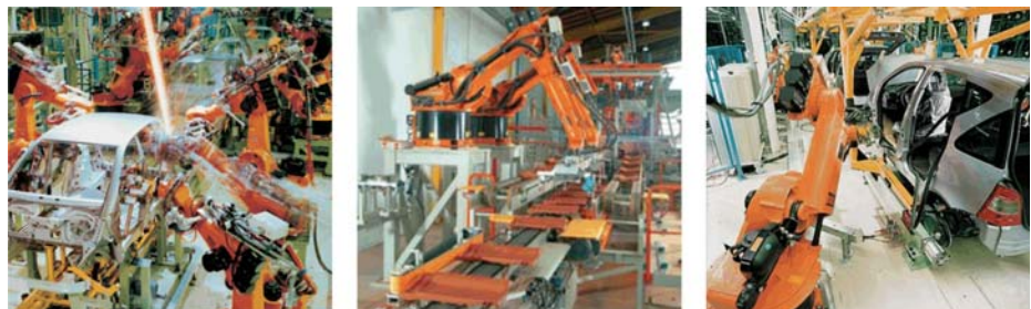
Figure 2: Modern industrial robots performing typical manufacturing tasks: spot welding, material handling and assembly [KUKA 2009].
