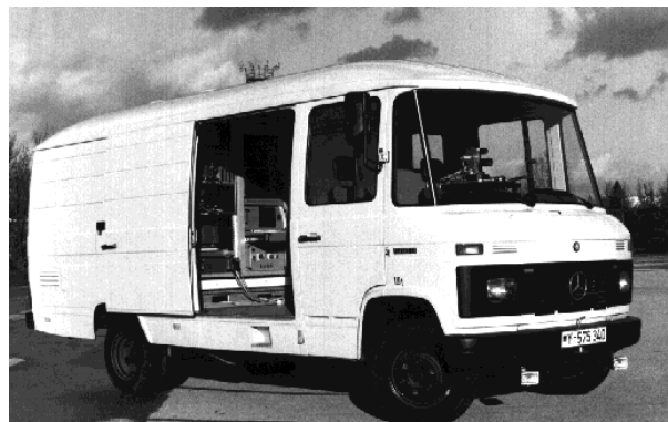
Figure 6: Autonomous road vehicle able to follow a road at a record speed of 96 km/h in 1987
