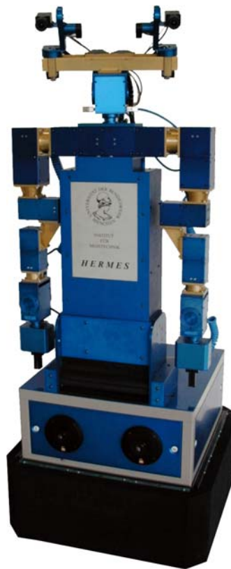
Figure 8: Humanoid experimental robot HERMES ; mass: 250 kg; size: 1.85 m x 0.7 m x 0.7 m
