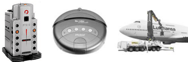
Figure 7: Typical service robots: mobile transportation robot Helpmate [King, Weiman 1990], vacuum cleaning robot Roomba [iRobot 2002], airplane cleaning robot Skywash [Schraft, Schmierer 2000]
