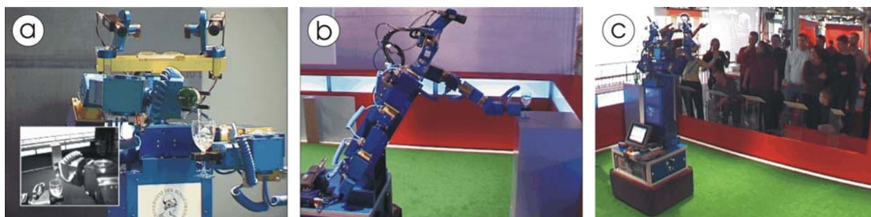
Figure 17: HERMES performing at the special exhibition "Computer.Brain", instructed by commands given in natural language by non-expert humans: taking over a bottle and a glass from a person (not shown), filling the glass with water from the bottle (a); driving to, and placing the filled glass onto, a table (b); interacting with visitors (here: waving with both arms, visitors wave back!) (c)
