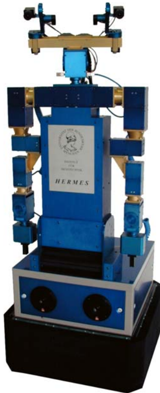
Figure 1: Versatile personal robot assistant HERMES ; size: 1.85 m x 0.7 m x 0.7 m; mass: 250 kg. The black material covering the undercarriage on all 4 sides is plastic foam that serves as a protective bumper and as part of an imaging tactile sensor.
