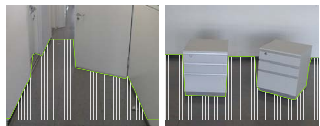
Figure 8: Gradient filtering along vertical search paths yields contour points that mark the transition between the floor and other objects. Left: typical corridor image with an open door as a possible obstacle. Right: two tables as possible docking objects.
