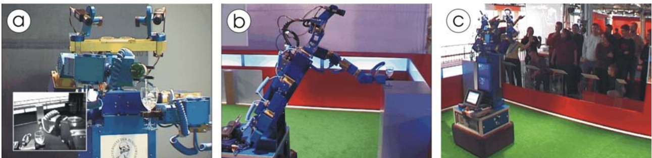
Figure 14: HERMES performing at the special exhibition “Computer.Brain”, instructed by natural language commands: taking over a bottle and a glass from a person (not shown), filling the glass with water from the bottle (a); driving to and placing the filled glass onto a table (b); interacting with the visitors (here: waving with both arms, visitors wave back!) (c)
