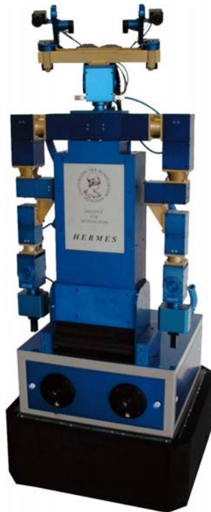
Figure 5 Versatile personal robot assistant HERMES ; size: 1.85 m x 0.7 m x 0.7 m; mass: 250 kg.
