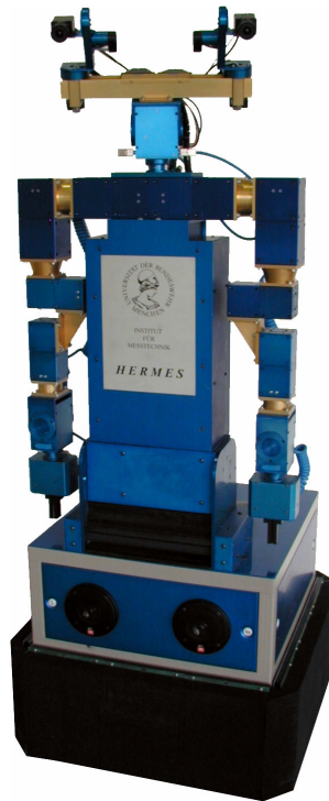
Figure 1: Humanoid experimental robot HERMES ; 1.85 m x 0.7 m x 0.7 m; mass: 250 kg
