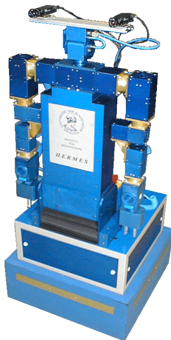
Figure 9: The humanoid robot HERMES with an omnidirectional wheel base, two arms with 6 degrees of freedom each and a stereo-vision system on a pan-tilt head; dim.: 70 cm x 70 cm x 170 cm.
