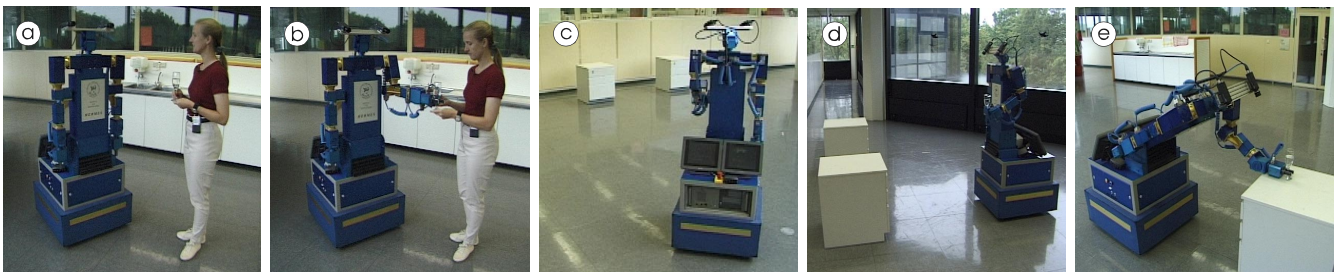
Figure 7: HERMES performing a simple service task upon user request: a) greetings and receiving first instructions (via a wireless microphone); b) receiving a glass from the user using kinesthetic sensing; not shown: further conversation with the user as to what to do next (see text); c) and d) approaching left table using a visual servoing method; e) placing glass onto the table.
