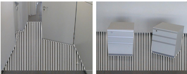
Figure 4: Gradient filtering along vertical search paths yields contour points that mark the transition between the floor and other objects. Left: typical corridor image with an open door as a possible obstacle. Right: two tables as possible docking objects.
